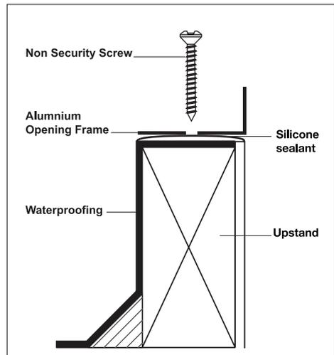
**IMPORTANT:** The overall upstand size must be 60mm smaller than the overall rooflight size (stated on rooflight packaging). (See CO1 for Constructing a Timber Upstand Curb), and internally must be 160mm smaller than overall rooflight size.
